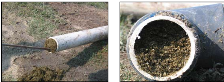
Figure7. Images of solid build up in PVC lines.
