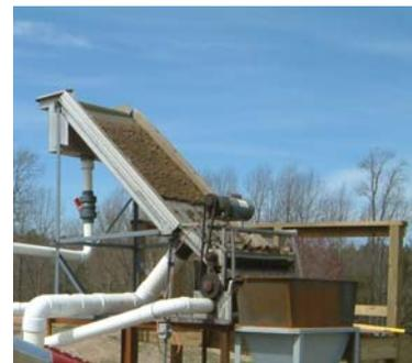
**Figure 2. Inclined Separator for Separating Raw Waste**
