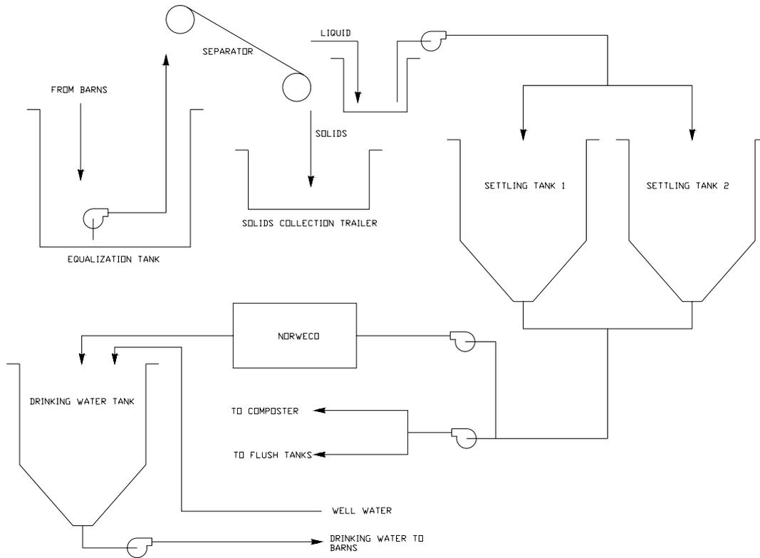
**Figure 1. System Schematic for “Closed-Loop” Swine Waste Treatment System**
