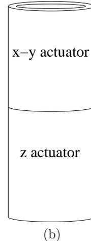
**Figure 2.** Actuator configurations employed for sample positioning in AFM. (a) Stacked actuators employed as  $x$ - and  $y$ -stages, and (b) cylindrical PZT transducer.
