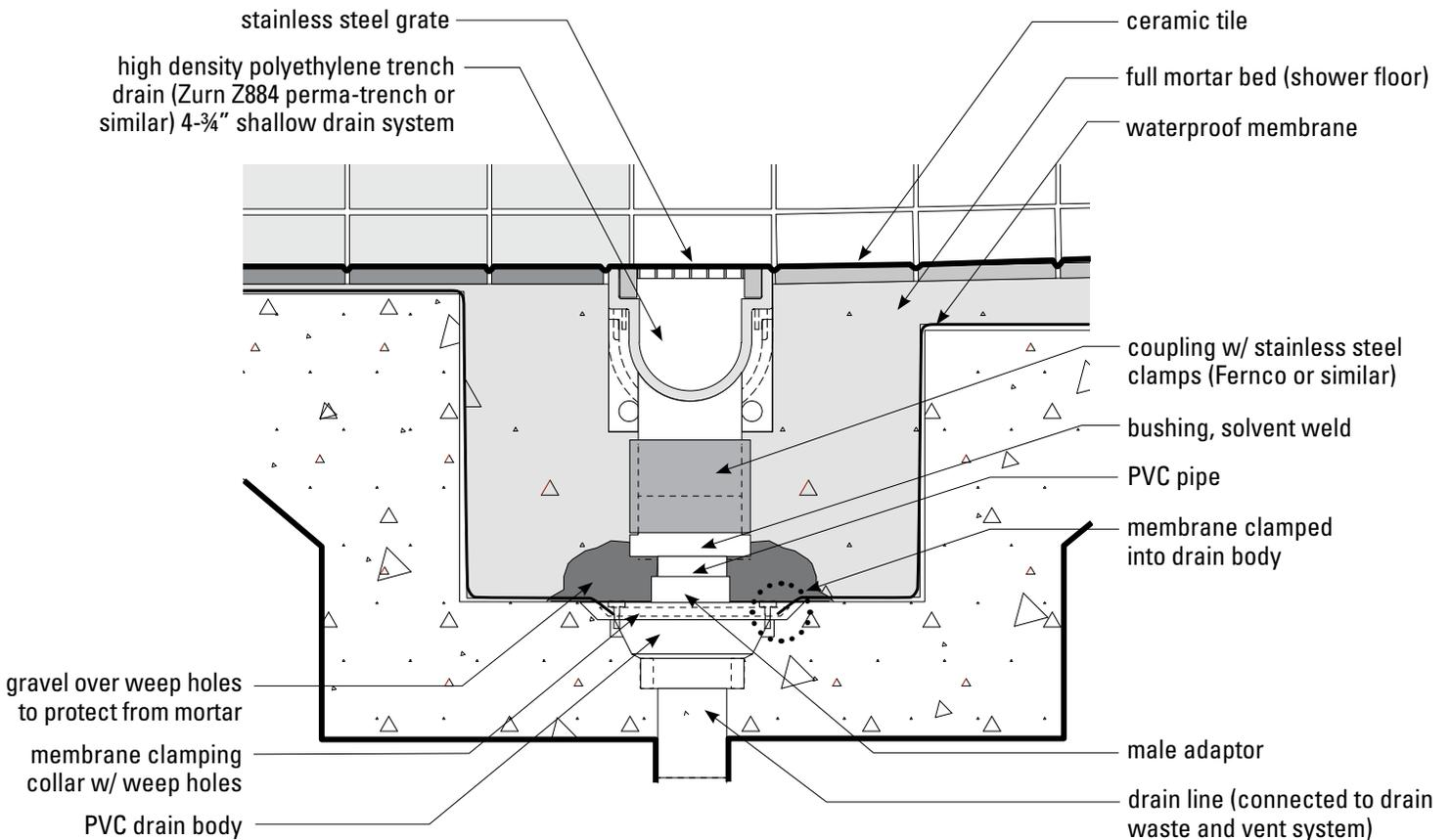
**Suggested Detail: Concrete Slab**
