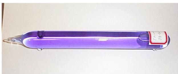
**Discussion:** Thionin is a common staining agent used in various biological applications. In this reaction, thionin (shown below) is photochemically reduced by  $\text{Fe}^{2+}$  in acidic conditions. This reaction is reversible as demonstrated in the absence of light. The following chemical reaction illustrates the reactivity observed:
