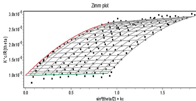
**Figure 1.** Typical Zimm plot by light scattering photometry from a Norway spruce lignin solution in THF.
