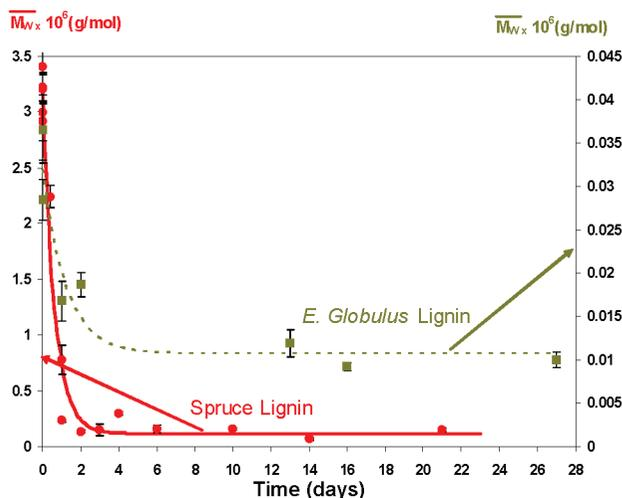
**Figure 7.** Incubation effect on the weight-average apparent molecular weight of the Norway spruce and *Eucalyptus globulus* lignin in THF solution maintained at room temperature.
