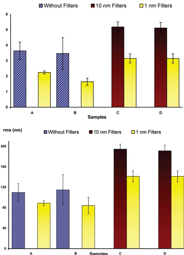
**Figure 2.** Effect of light scattering filters on the weight-average apparent molecular weight (top graph) and on the root-mean-square radius (bottom graph) of EMAL Norway spruce solutions in THF.
