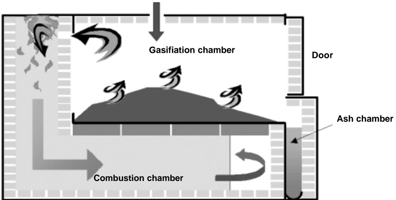
**Figure 1. Diagram of the BGP gasifier.**
