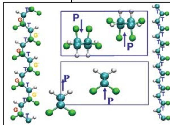
This diagram shows the difference between polarized and non-polarized PVDF molecules. The non-polarized molecules (top box) produce the polymer chain on the left, while the chain on the right is produced by the polarized molecules (bottom box).
