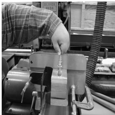
Figure 6. – Belt sander with specimen and weight.
