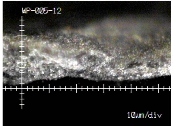
Figure 4. – Blade used to cut ChoiceDek material after 125 feet of cutting.
