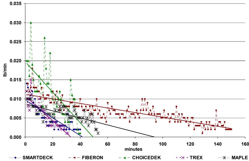
Figure 7. – Material removal rates (lb/min) for various specimens against time. The trendlines are calculated using least square regression.
