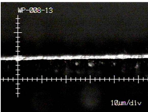
Figure 5. – Blade used to cut with pine after 125 feet of cutting.
