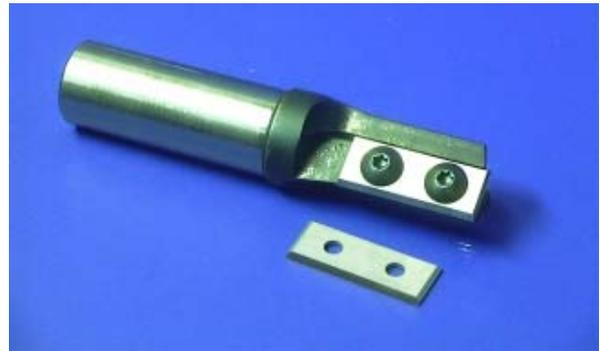
Figure 2. – Carbide insert and tool holder
