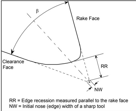
Figure 1. – Determining knife wear by measuring the nose width (NW) after each test cycle.
